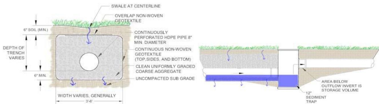
Figure 3: Infiltration Trench Diagram
